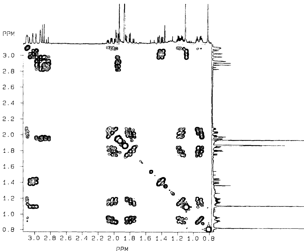
Figure. High-field region of COSY plot of (-)-4. After Fourier transformation, the absolute-value spectra was folded and represented as a contour plot.
